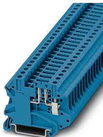
Disconnect terminal block, With test socket screws for insertion of test plugs, nom. voltage: 500 V, nominal current: 20 A, connection method: Screw connection, cross section: 0.14 mm<sup>2</sup> - 6 mm<sup>2</sup>, AWG: 26 - 10, length: 57.8 mm, width: 6.2 mm, color: blue, mounting: NS 35/7,5, NS 35/15
